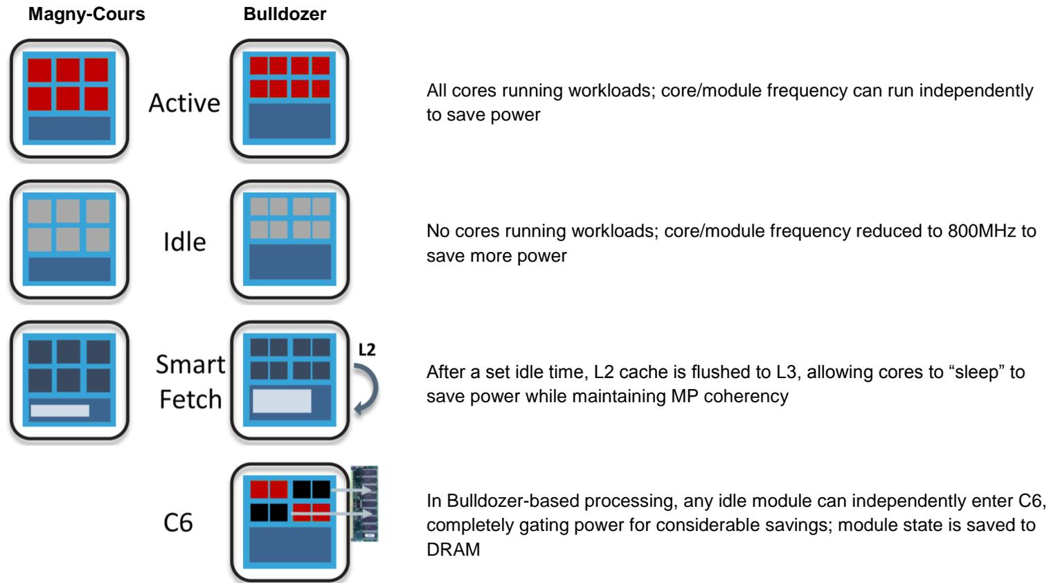
The new C6 power state reduces processor power consumption at idle by up to 46%.
