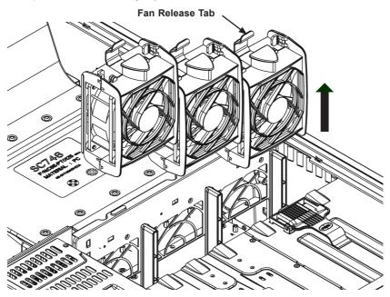
Figure 5-23: Front Chassis Fans
