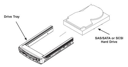
Figure 5-14: Removing the Dummy Drive Tray
