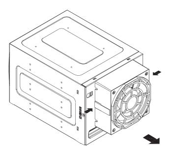
Figure C-5: Removing Mobile Rack Fan
