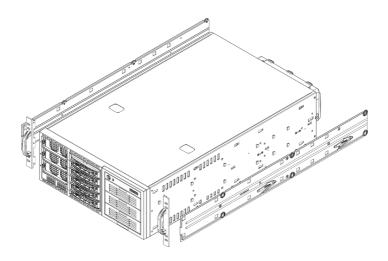
Figure 6-4: Installing the Inner Rack Rails
