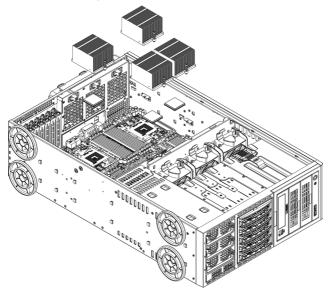
Figure 5-18: Installing Heatsinks
