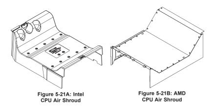
Air shrouds concentrate airflow to maximize fan efficiency. The SC748 chassis air shroud does not require screws to set it up.
