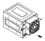
Figure D-6: Removing the Exhaust Fan
