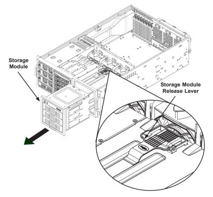
Figure 5-4: Remove the Storage Module
