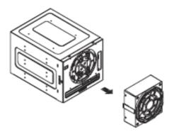
Figure D-7: Pulling Off the Exhaust Fan
