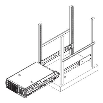
Figure 6-7: Installing the Chassis into a Rack
