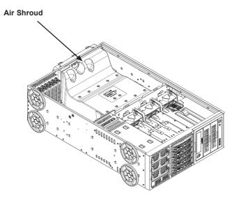
Figure 5-22: Air Shroud in Place
