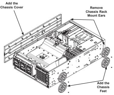
Figure 6-8: Adding Chassis Feet and Top Cover Installing the Chassis Cover
