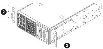
Figure 6-3: Identifying the Inner Rails and Chassis Handles
