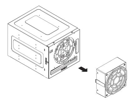
Figure C-6: Removing Mobile Rack Fan
