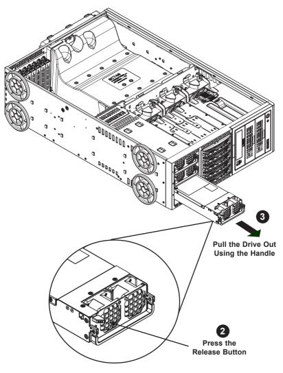
Figure 5-25: Removing a Power Supply
