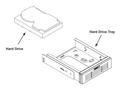
Figure 5-7: Add a Hard Drive to the Drive Tray
