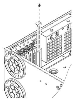
Figure 5-20: Remove PCI Card Slot Guard
