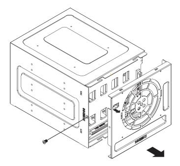
Figure C-7: Removing Mobile Rack Fan
