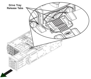
Figure 5-10: Removing the Drive Bay
