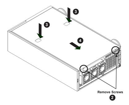
Figure 5-1: Removing the Chassis Cover
