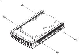
Figure 5-15: Installing the Hard Drive
