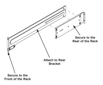
Figure 6-5: Assembling the Outer Rails
