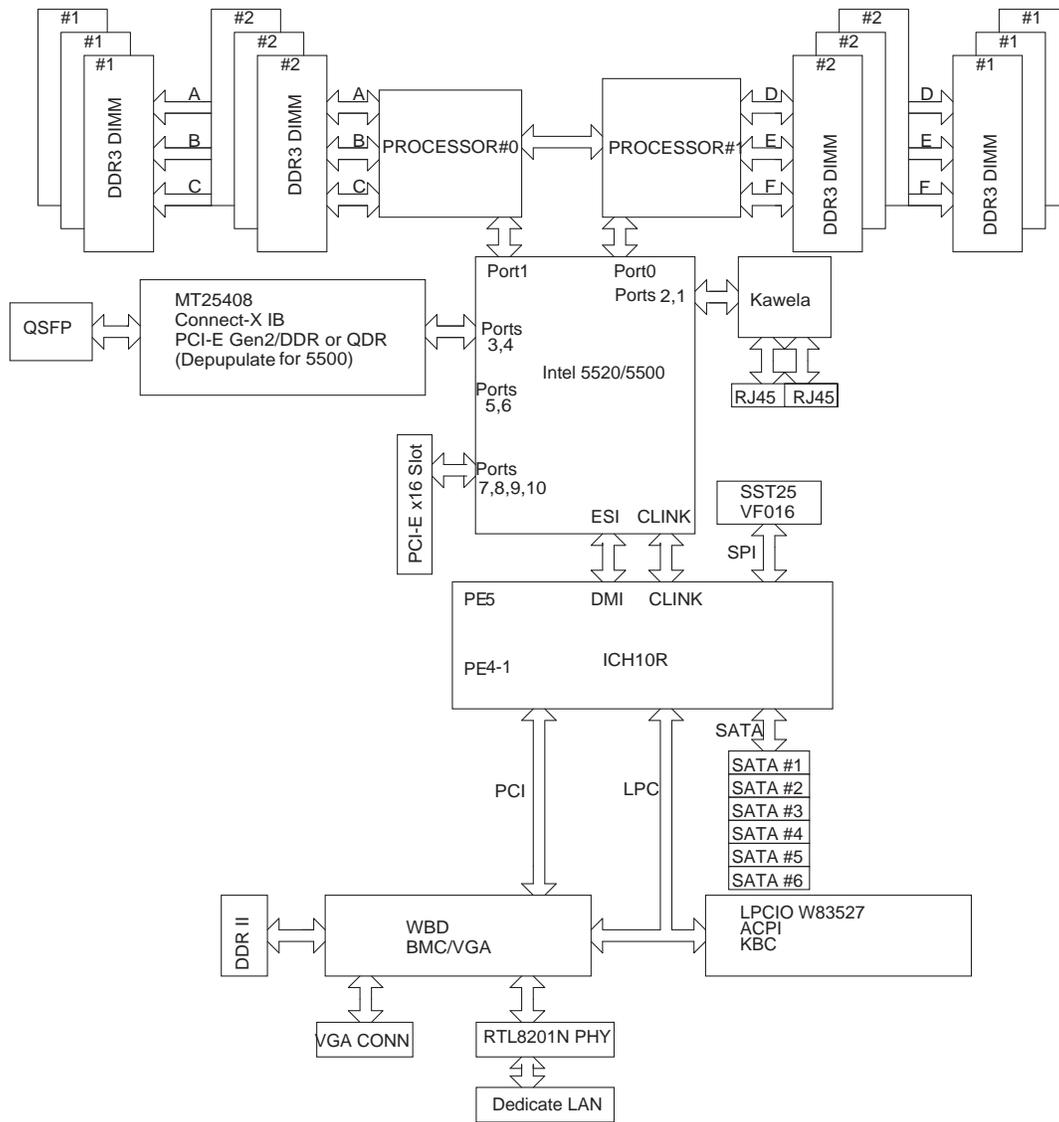
**Block Diagram of the 5500/5600 Series Processor Platform**
