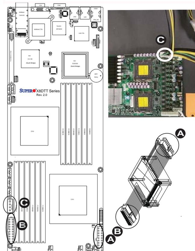
A. Right 20-pin PWR connector & cable: (PWR1)
