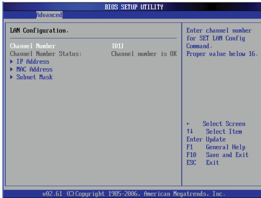
**Channel Number** - Enter the channel number for the SET LAN Config command. This is initially set to **[1]**. Press "+" or "-" on your keyboard to change the Channel Number.
