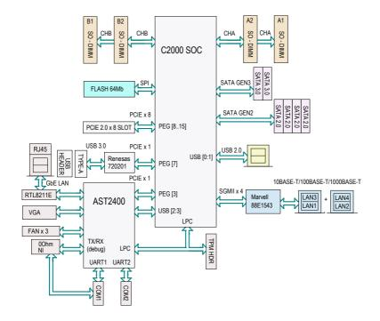
A1SAi & A1SRi Series motherboard Block Diagram
