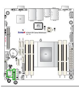
A. Internal Buzzer B. PWR LED/ Speaker Header
