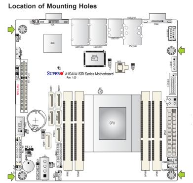
**Caution:** 1) To avoid damaging the motherboard and its components, please do not use a force greater than 8 lb/inch on each mounting screw during motherboard installation. 2) Some components are very close to the mounting holes. Please take precautionary measures to avoid damaging these components when installing the motherboard to the chassis.
