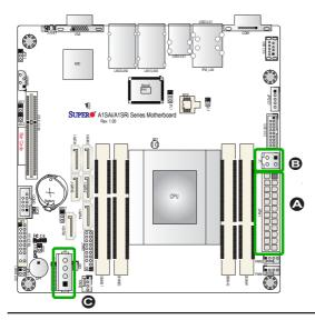
A. 24-Pin ATX PWR B. 4-Pin 12V DC Alternative Power Source (up to 144W) C. 4-Pin HDD PWR
